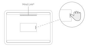
\* Press to open the magnetic cover to replace the SSD drive.
