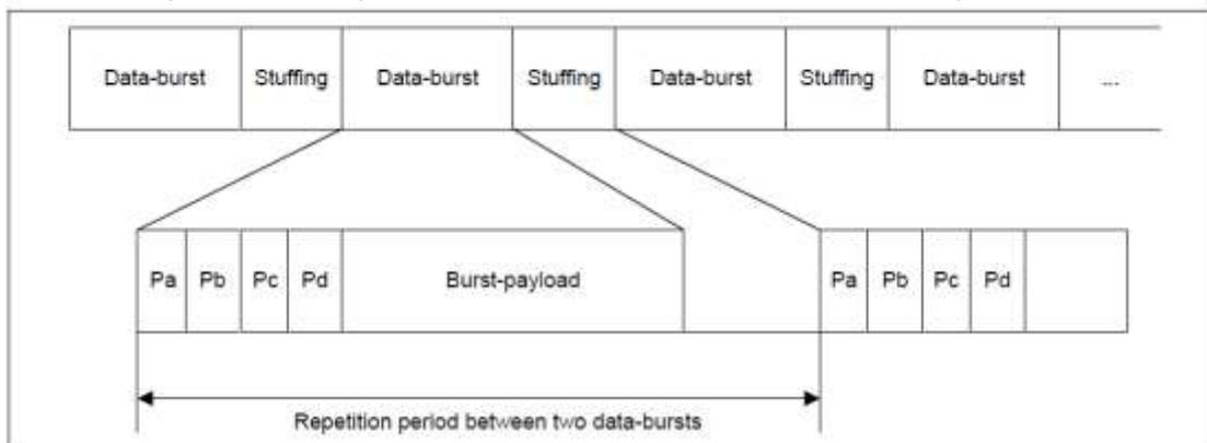
Fig. 24-6 Format of Data-burst
