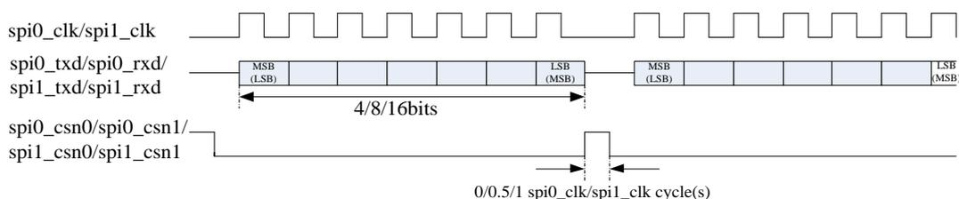
Fig. 23-5 SPI Format (SCPH=1 SCPOL=0)
