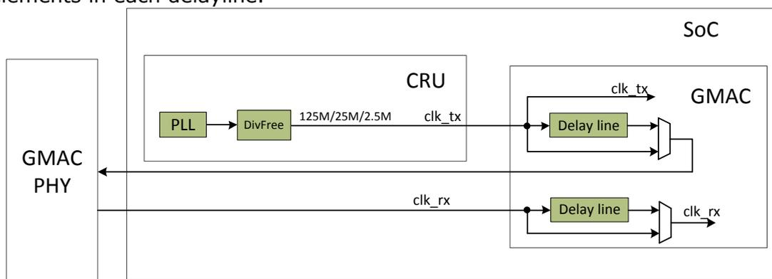
Fig. 25-14 RGMII clock architecture when clock source from CRU
