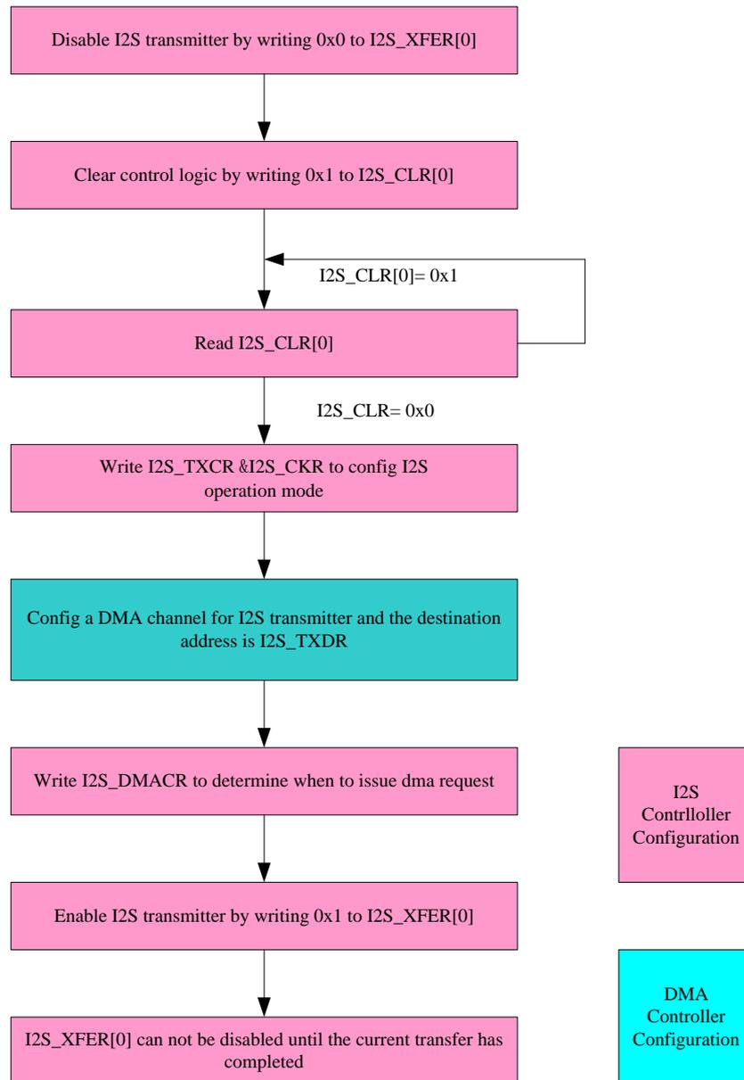
Fig. 22-11 I2S/PCM controller transmit operation flow chart
