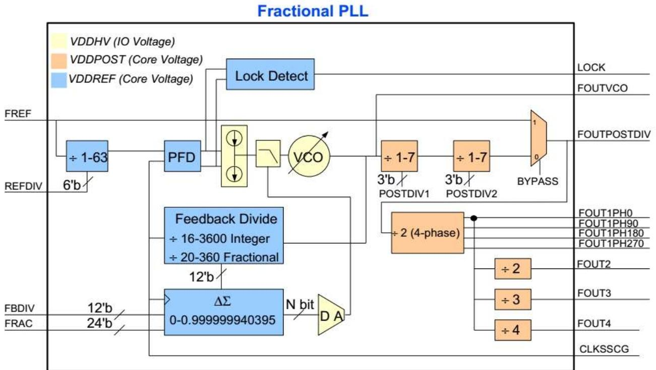
Fig. 2-6 PLL Block Diagram
