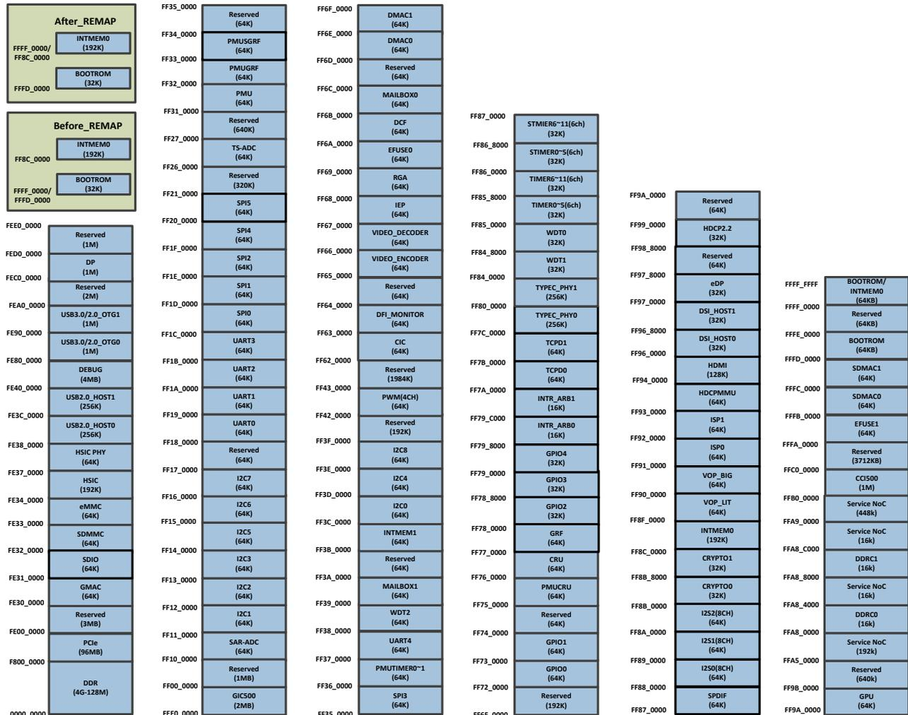
Fig. 1-1 RK3399 Address Mapping
