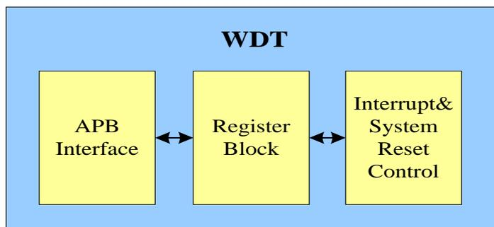
Fig. 17-1 WDT block diagram
