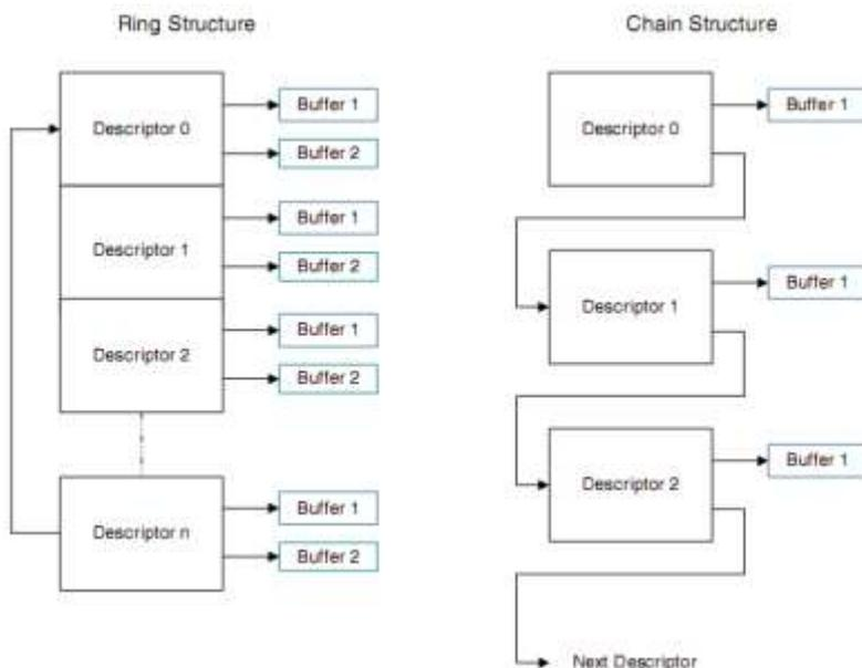
Fig. 25-10 Descriptor Ring and Chain Structure
