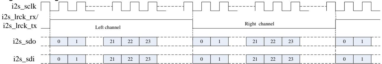
Fig. 22-5 I2S left justified mode timing format
