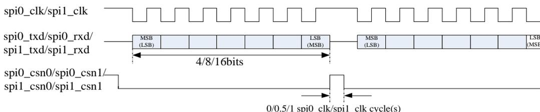
Fig. 23-6 SPI Format (SCPH=1 SCPOL=1)
