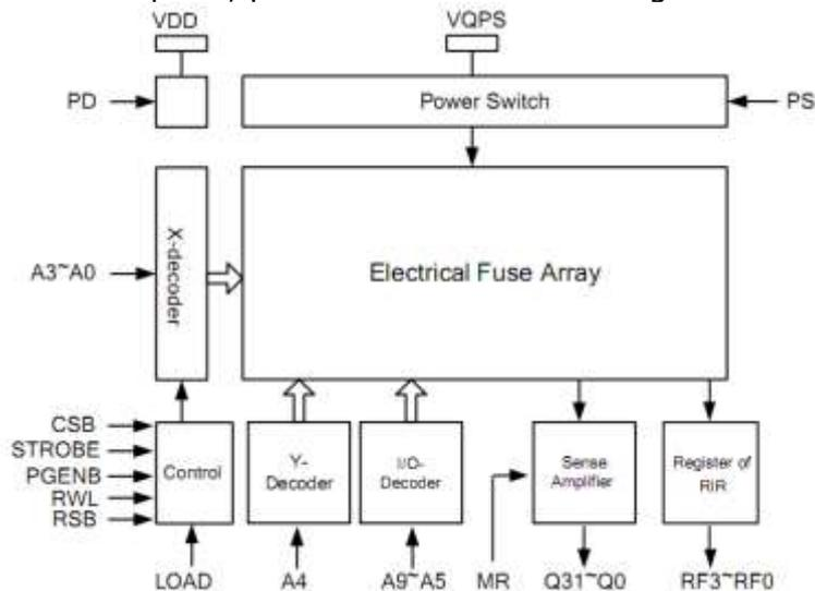
Fig. 16-1 eFuse block diagram
