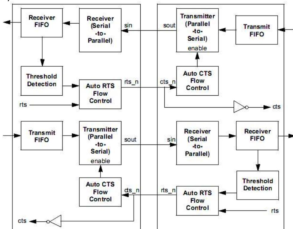
Fig. 19-5 UART Auto flow control block diagram
