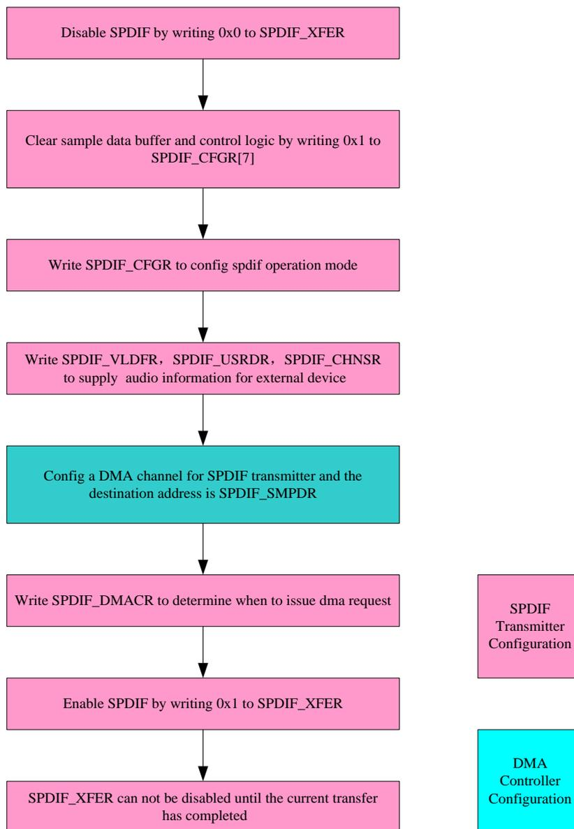
Fig. 24-7 SPDIF transmitter operation flow chart
