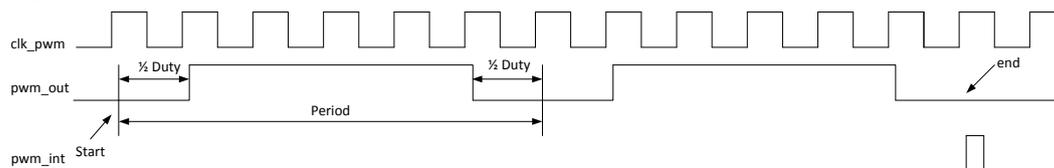
Fig. 18-5 PWM One-shot Center-aligned Output Mode
