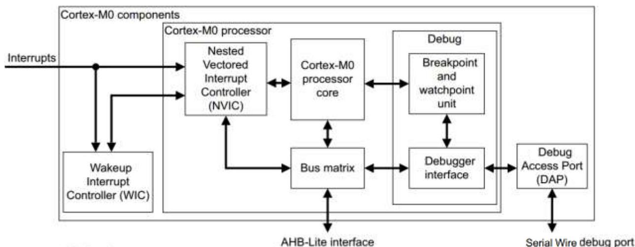
Fig. 6-1 Cortex-M0 Integration Architecture
