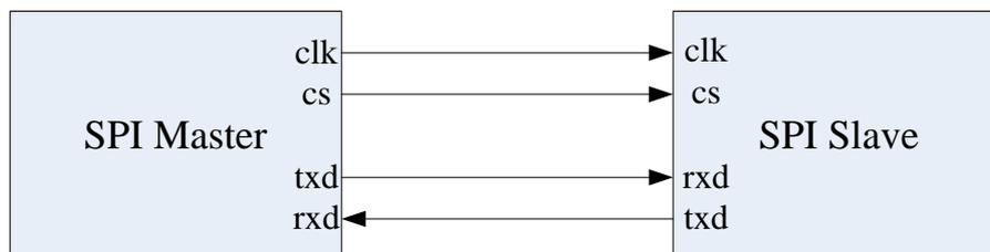
Fig. 23-2 SPI Master and Slave Interconnection
