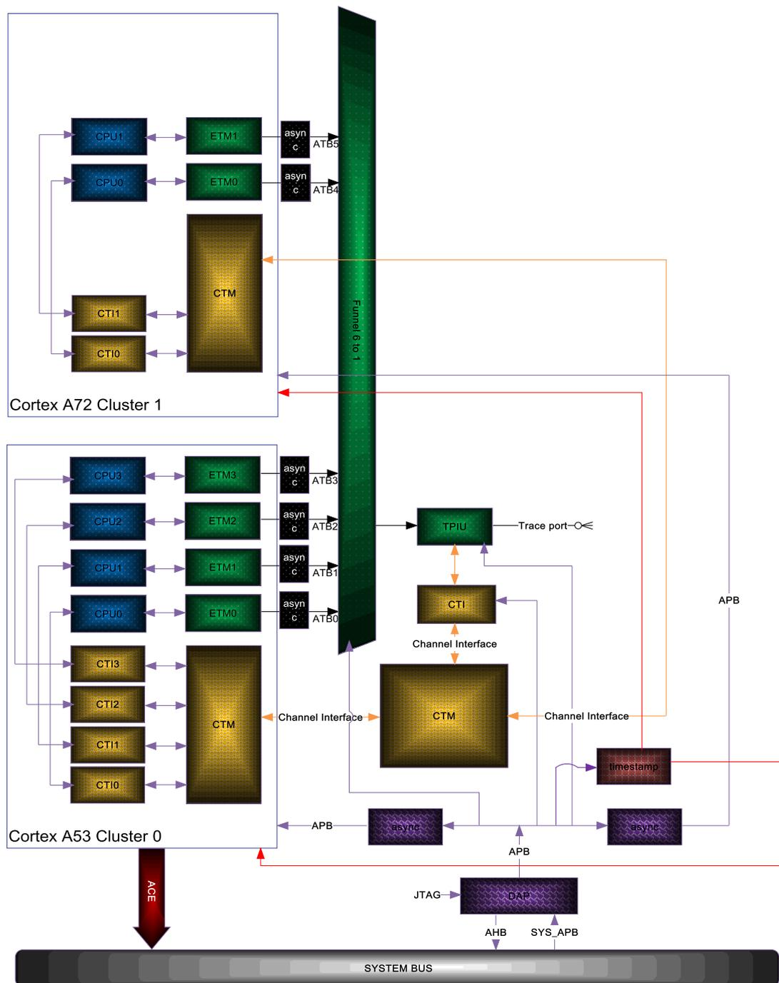
Fig. 14-1 RK3399 Debug system structure
