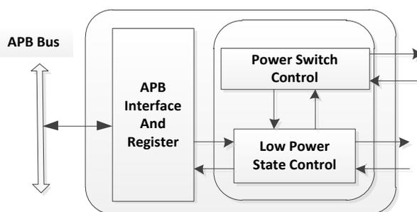
Fig. 8-2 PMU Bock Diagram
