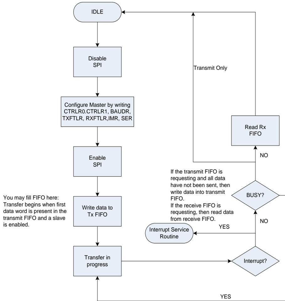
Fig. 23-7 SPI Master transfer flow diagram
