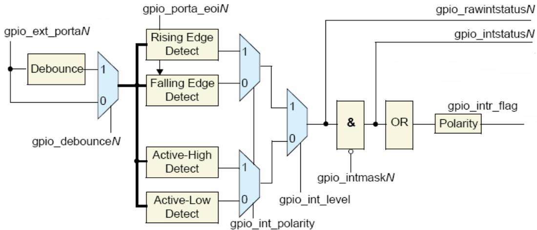
Fig. 20-2 GPIO Interrupt RTL Block Diagram
