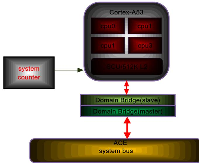
Fig. 5-1 Block Diagram
