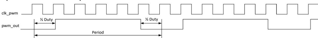
Fig. 18-4 PWM Continuous Center-aligned Output Mode
