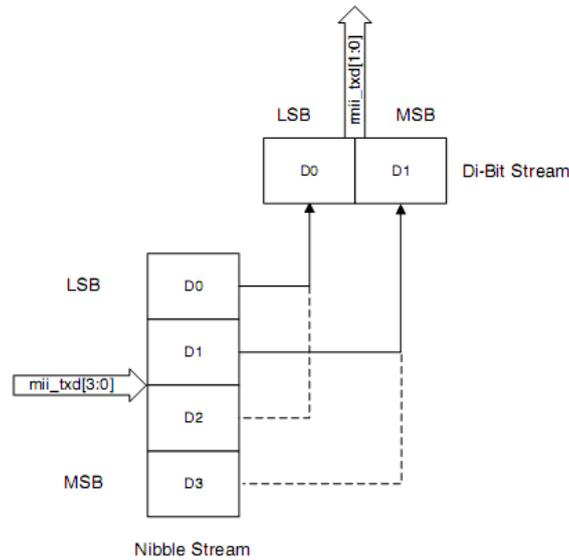
Fig. 25-3 RMII transmission bit ordering
