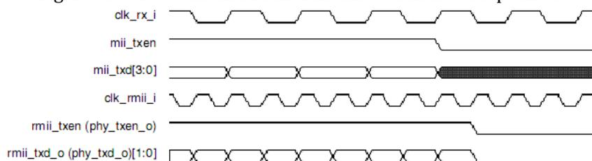
Fig. 25-5 End of MII and RMII Transmission in 100-Mbps Mode
