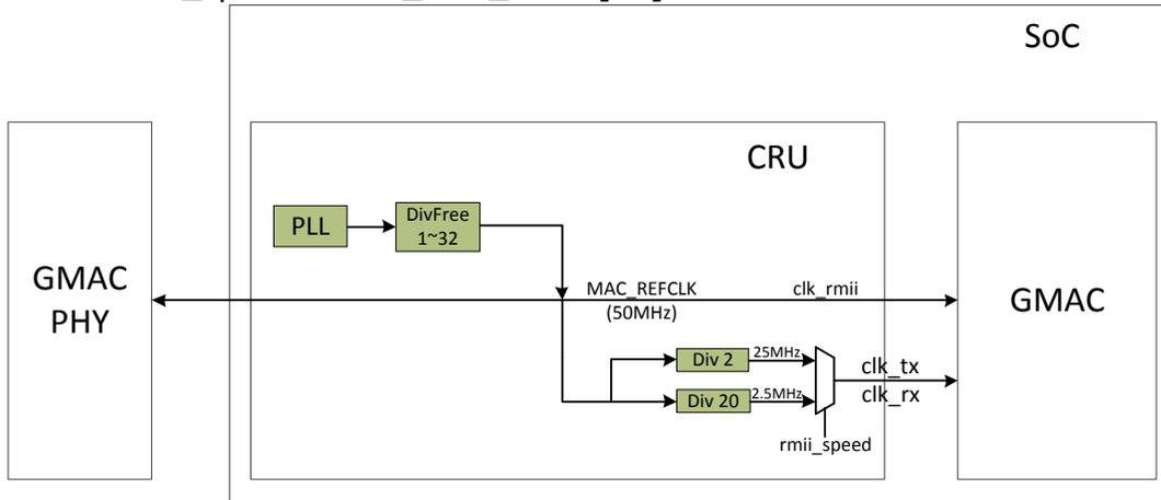
Fig. 25-12 RMII clock architecture when clock source from CRU
