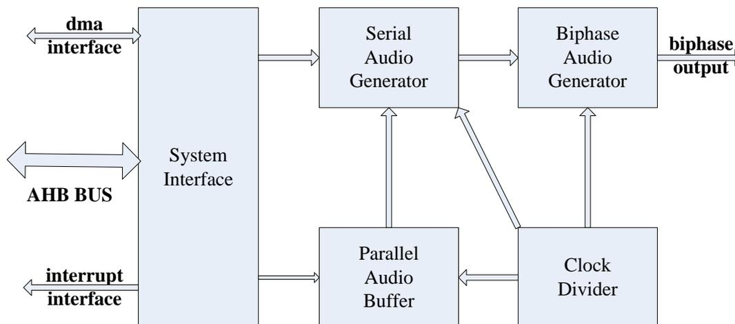
Fig. 24-1 SPDIF transmitter Block Diagram
