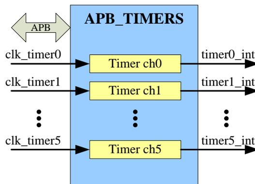
Fig. 10-1 Timer Block Diagram
