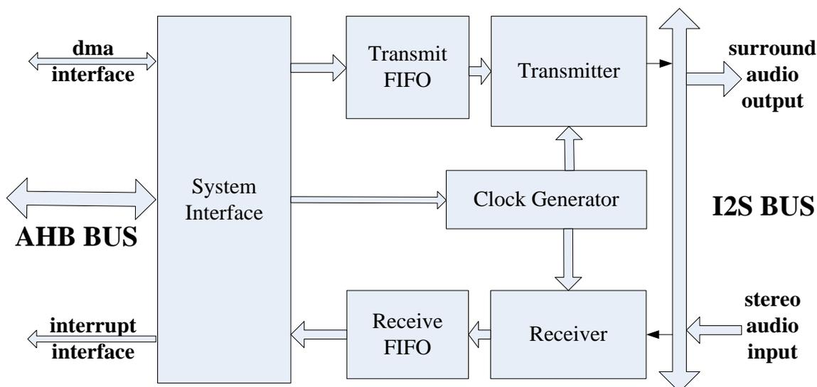
Fig. 22-1 I2S/PCM controller (8 channel) Block Diagram
