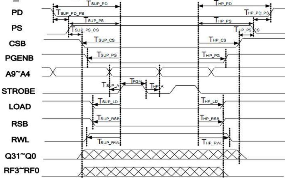
Fig. 16-3 eFuse timing diagram R\_PGM mode
