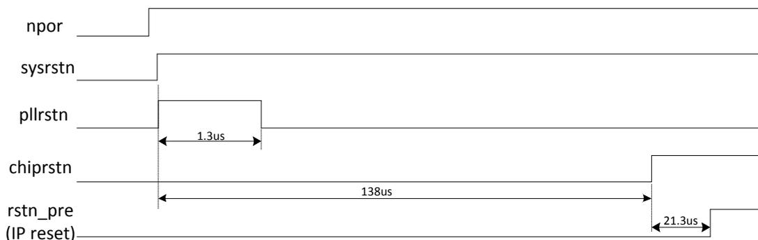
Fig. 2-7 Chip Power On Reset Timing Diagram
