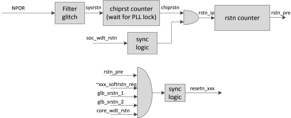
Fig. 2-5 Reset Architecture Diagram
