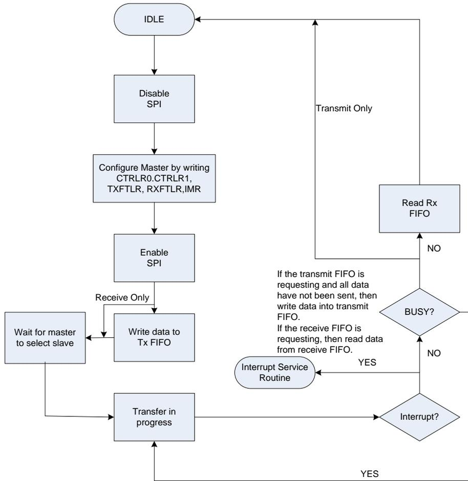
Fig. 23-8 SPI Slave transfer flow diagram
