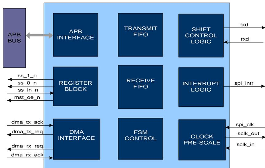
Fig. 23-1 SPI Controller Block diagram
