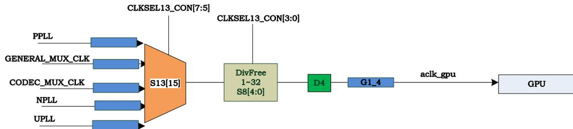
Fig. 27-2 ACLK\_GPU generate block diagram
