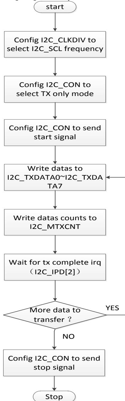
Fig. 21-6 I2C Flow chat for transmit only mode
