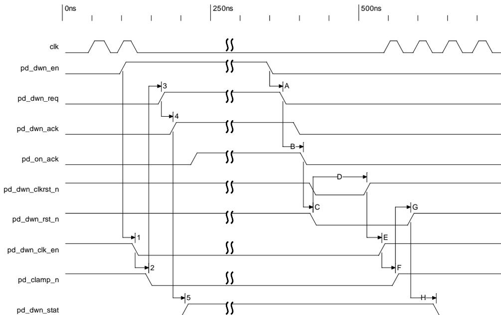
Fig. 4-5 Each Domain Power Switch Timing
