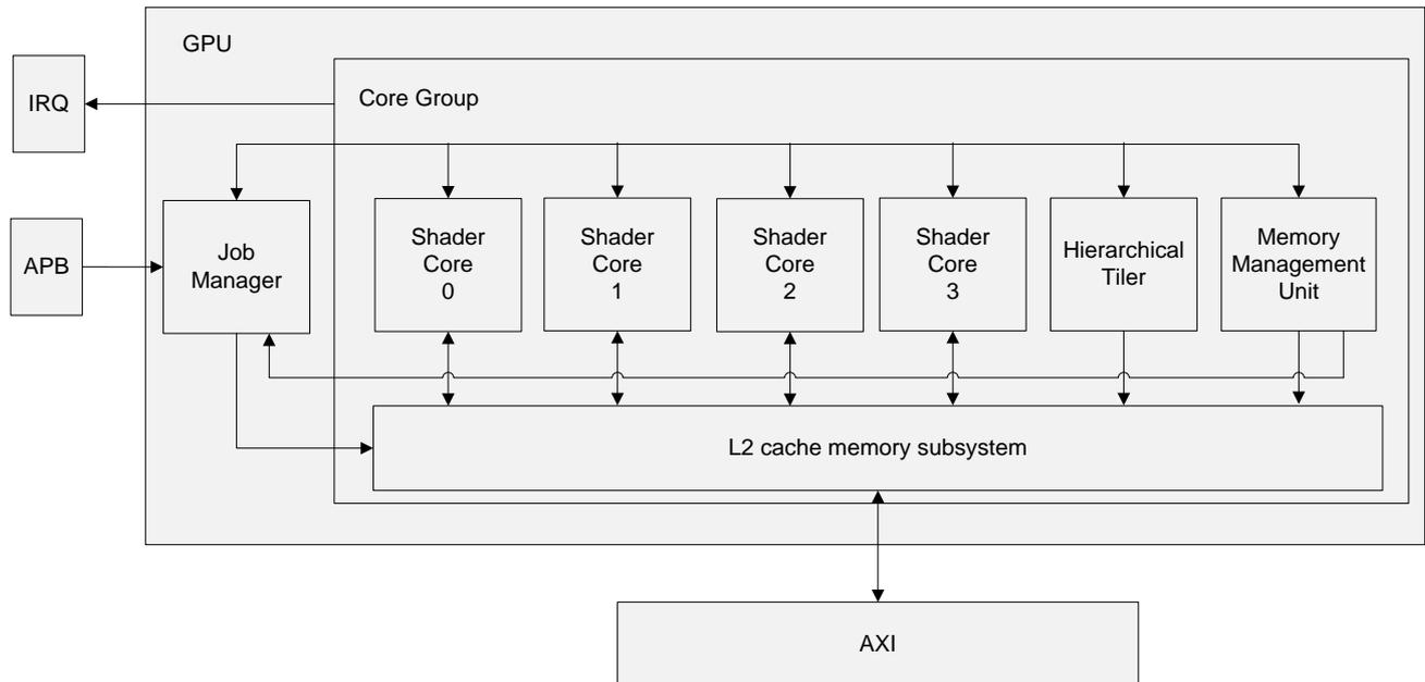
Fig. 27-1 GPU block diagram
