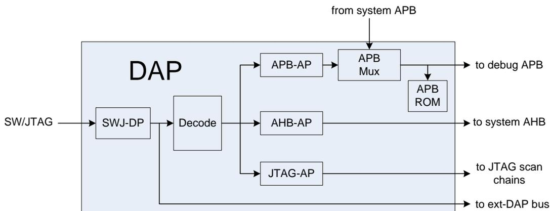
Fig. 14-2 RK3399 Debug system DAP structure
