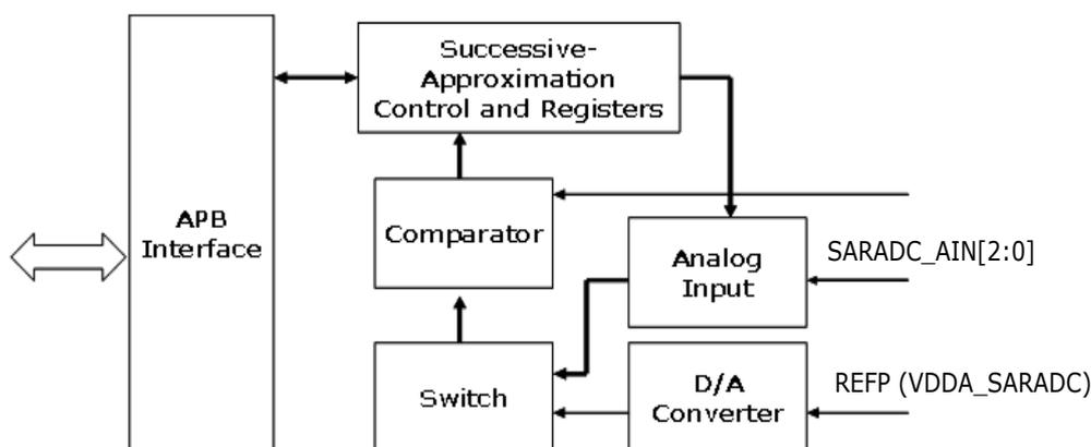
Fig. 26-1 RK3399SAR-ADC block diagram
