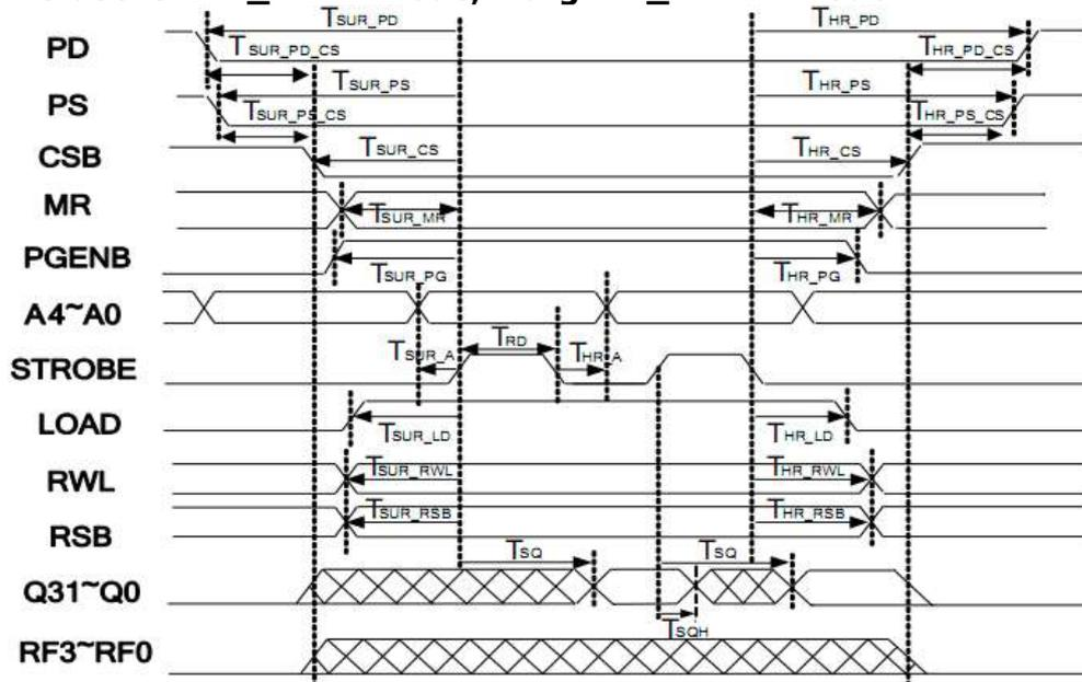
Fig. 16-4 eFuse timing diagram in A\_READ mode and Margin A\_READ1 Mode
