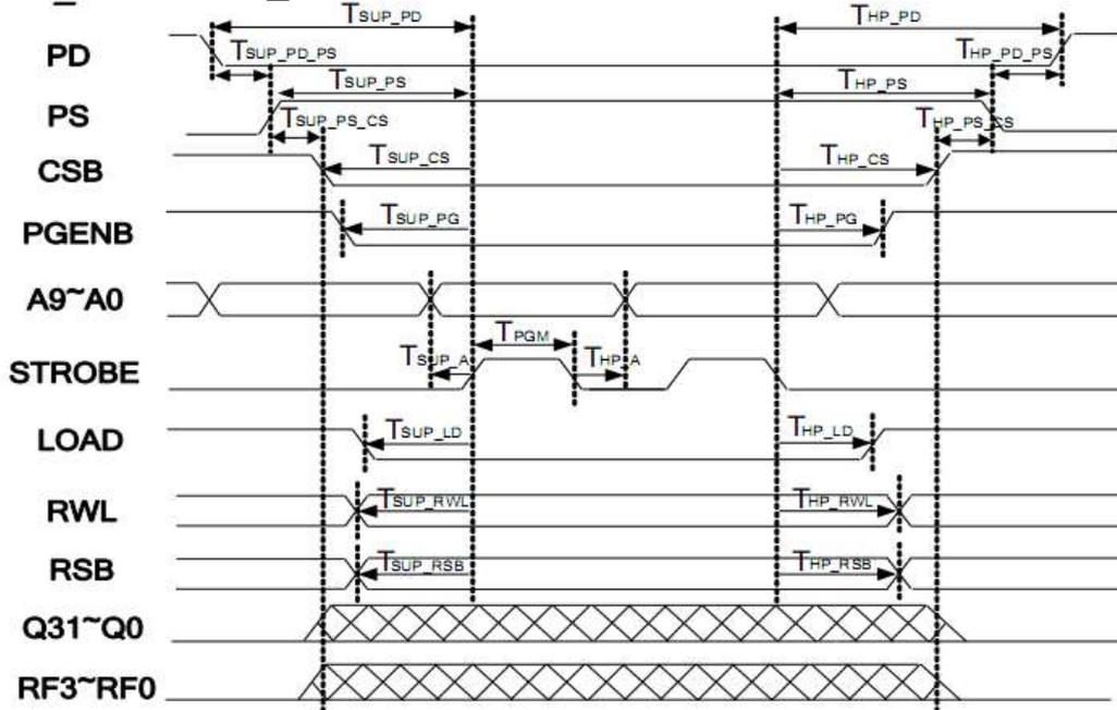
Fig. 16-2 eFuse timing diagram A\_PGM mode
