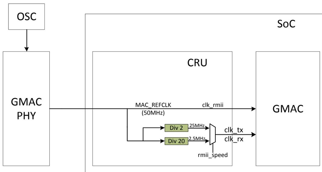
Fig. 25-13 RGMII clock architecture when clock source from external OSC
