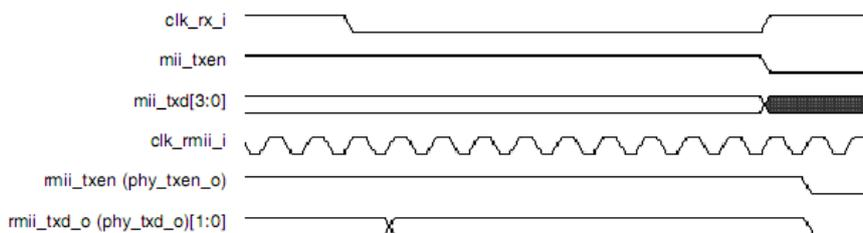
Fig. 25-7 End of MII and RMI Transmission in 10-Mbps Mode
