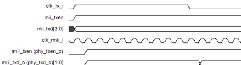
Fig. 25-6 Start of MII and RMII Transmission in 10-Mbps Mode
