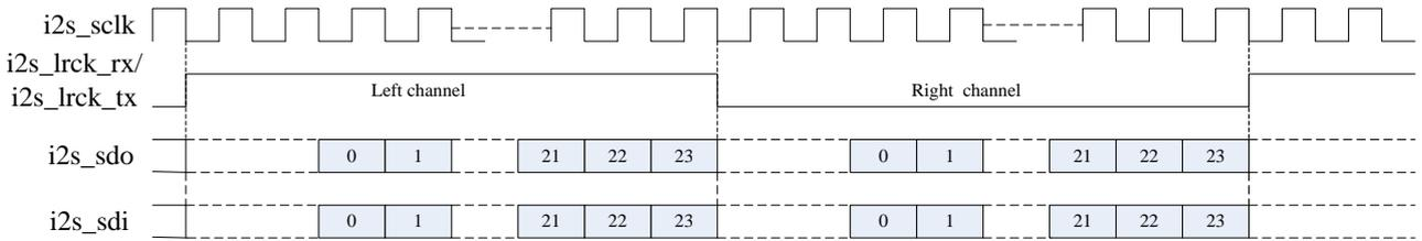
Fig. 22-6 I2S right justified mode timing format
