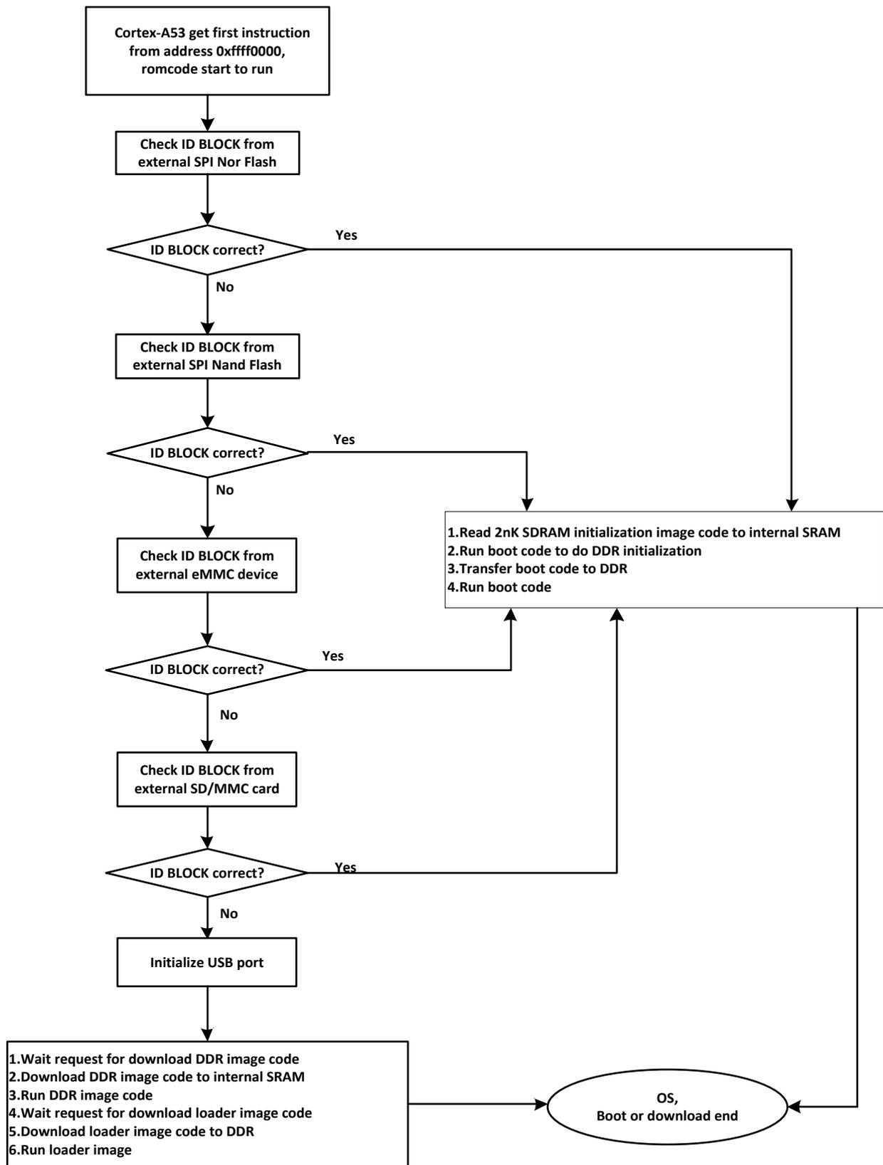
Fig. 1-2 RK3399 boot procedure flow
