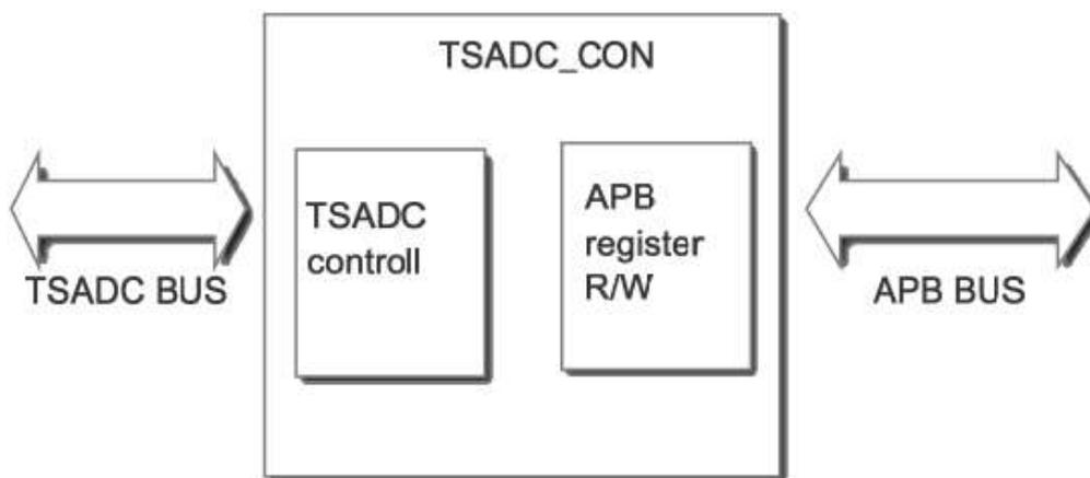
Fig. 13-1 TS-ADC Controller Block Diagram
