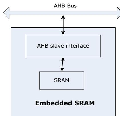
Fig. 7-1 8KB Embedded SRAM block diagram
