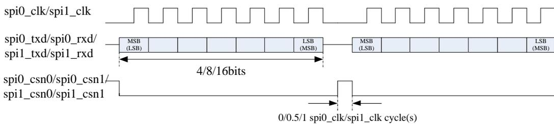
Fig. 23-3 SPI Format (SCPH=0 SCPOL=0)
