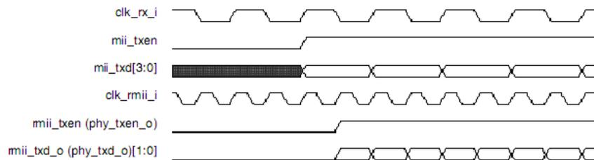
Fig. 25-4 Start of MII and RMII transmission in 100-Mbps mode
