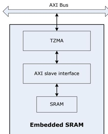
Fig. 7-2 192KB Embedded SRAM block diagram
