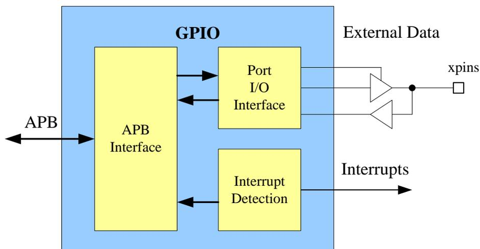
Fig. 20-1 GPIO block diagram
