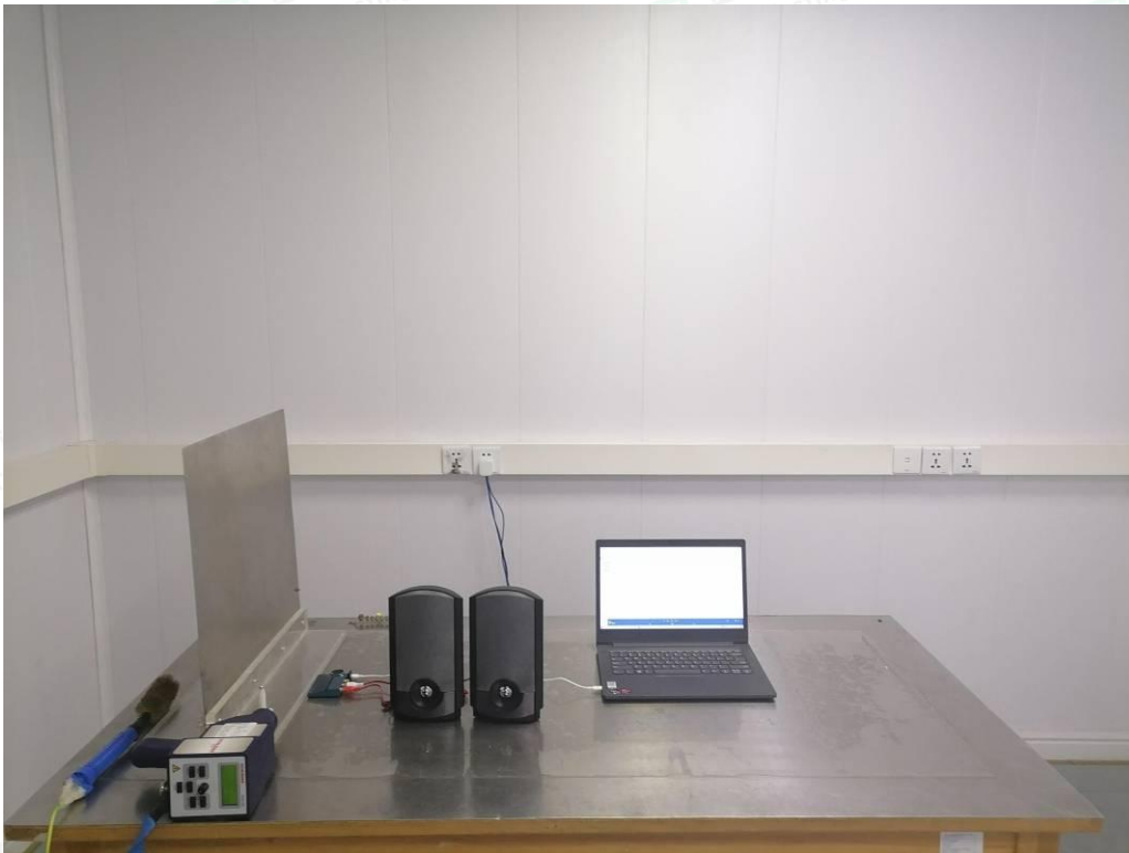
Test Setup Photo of Electrostatic Discharge Test
